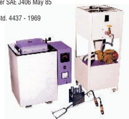
Jominy End Quench Hardenability Set-up
