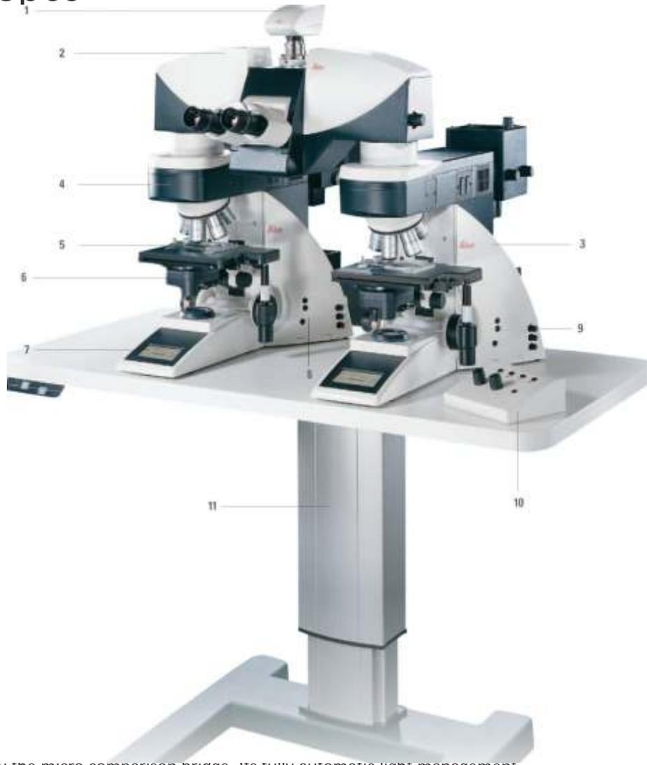
The Leica DM4000B complements perfectly the micro comparison bridge. Its fully automatic light management, integrated Variolux color module, selected optics pairs and reproducible illumination ensure you the greatest possible comparison reliability.
